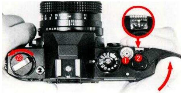
6. Turn the film transport lever until it does not move further and depress the Shutter Release Button (1). Repeat this action till the figure "1" comes in alignment with the index mark in the window of the Film Counter (2). If the film is transported in the correct manner when the film transport lever is turned, the Film Rewind Knob (23) will revolve counterclockwise. If it does not turn counterclockwise, rewind the film (see Page 50) and start all over again.
