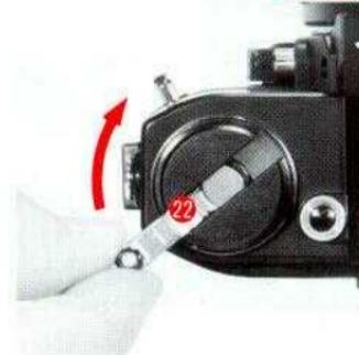
5. Flip up the Film Rewind Crank (22) and turn it in the direction indicated by an arrow mark on it to reduce the slack of the film.
