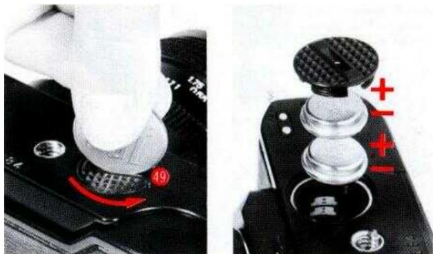
1. Turn the cover of the Mercury Battery Chamber (49) counterclockwise with a coin or something alike and detach it from the chamber.
