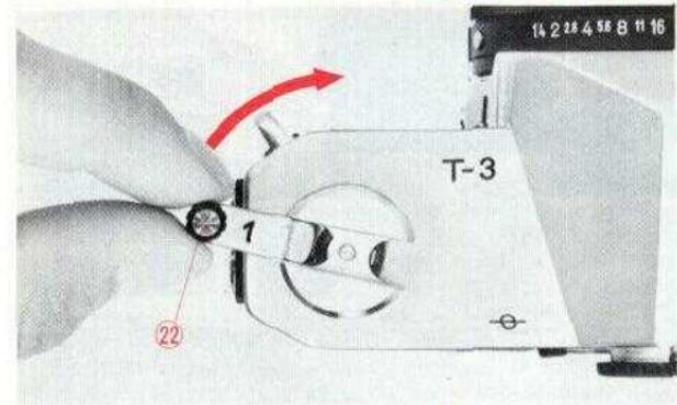
4. While lightly pressing down the cartridge, turn the Film Wind Lever (14) and take up the film on the spool. Ascertain that the teeth of the Sprocket (35) are in gear with film perforations before the back cover is closed. Depress the back cover with a finger tip, and it will be closed with ease.
