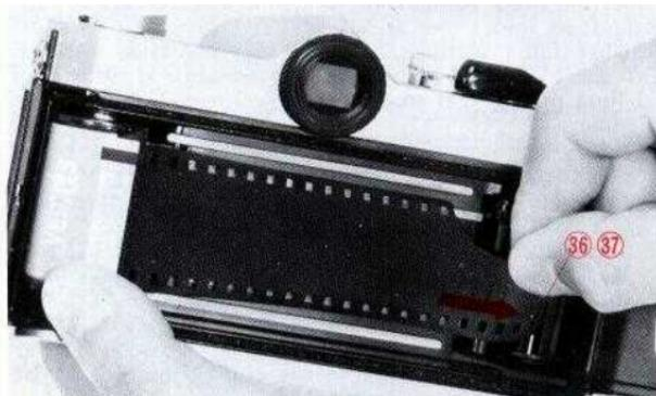
1. Pull the Back Cover Lock (28) and open the Back Cover (39).
