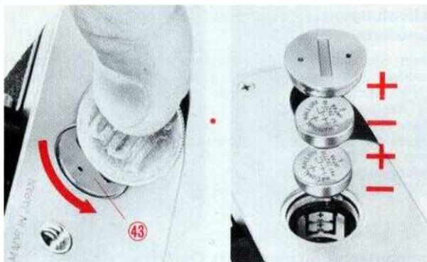
The KONICA Autoreflex-T3's TTL meter takes two 1.35V mercury batteries as its electric source. Wipe the separately enclosed mercury battery cells with a piece of dry and clean cloth and put them into the mercury battery chamber.
