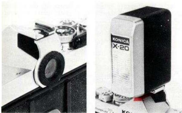
**1. Mount the Hot Shoe Clip:** Turn the frame of the eyepiece assembly counterclockwise and take it off. Place the hot shoe clip and the frame on it. Tightly screw the frame in on the frame clockwise. The conventional KONICA Accessory Clip 3 may also be fixed and used.
